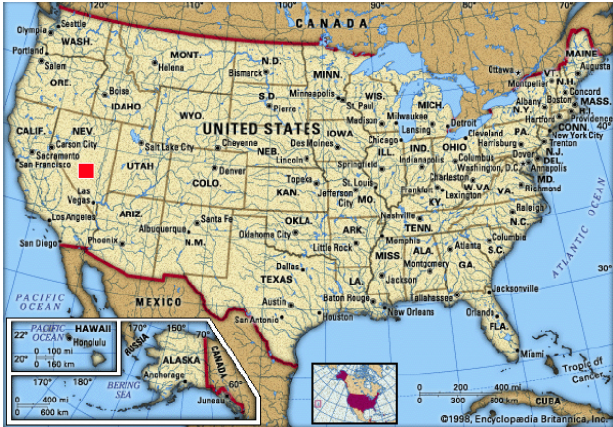
Figure 1-1. Area (in red) covered with 15% efficient solar cells could provide a years woth of electricity for the US
